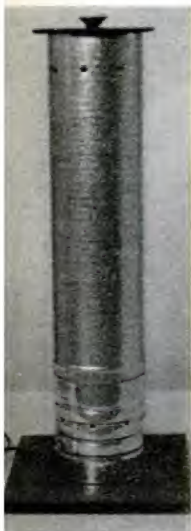
SIMPLE FILM DRYER using a 40-watt light bulb will dry negative strips dust-free in half an hour. The base is a one-gallon tin can and the chimney is a two-foot length of six-inch galvanized stovepipe. Drill \frac{1}{2} -inch holes around the can and the top of the pipe. Air
